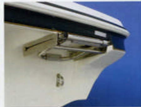
A hidden ladder makes boarding the boat easy. Tucked under the integrated swim platform, it's easier to reach, and there's nothing to trip over while standing on the platform.
