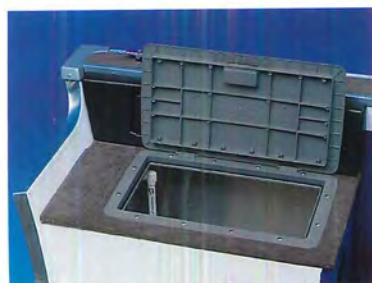
Live well with recirculating pump
