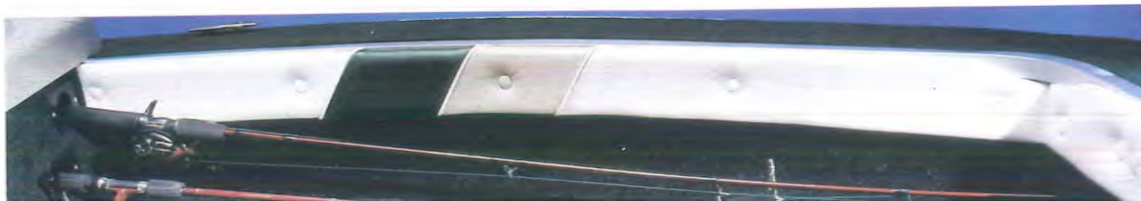
Redesigned stern with extra storage space, livewell and seat base.
