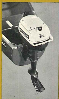
Photo showing secure attachment of motor to stern of canoe.
