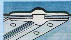
Standard Canoe Cross Section of Standard Canoe keel, an inner-outer heat treated extrusion riveted to the canoe hull.
