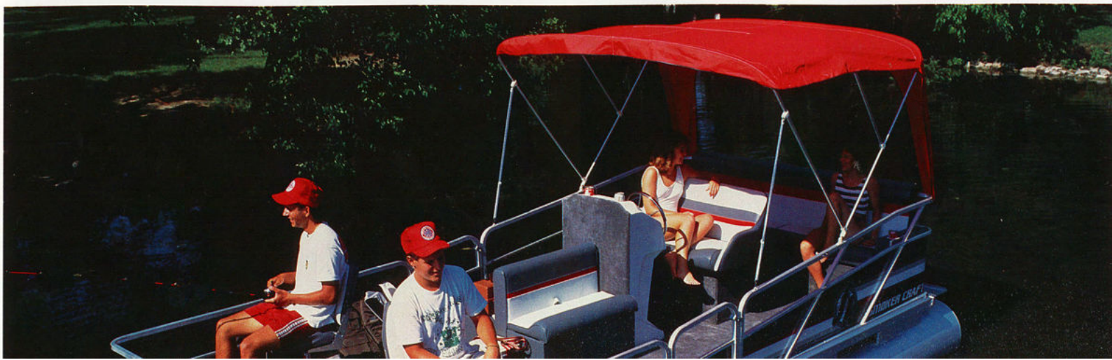
161 Magnum Length: 16'2" Beam: 76" Horsepower: 80 Weight: 700 Capacity: 1400
