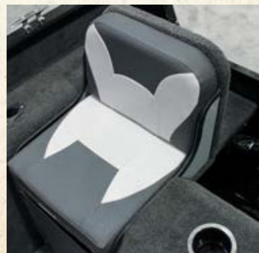
FLIP-UP JUMP SEAT OPTIONAL | convert from a spacious casting deck to additional passenger seating at the stern
