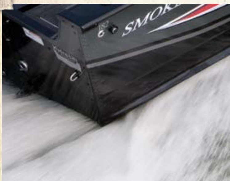
INTEGRATED SPRAY RAIL | pushes water away from the hull for a drier ride
