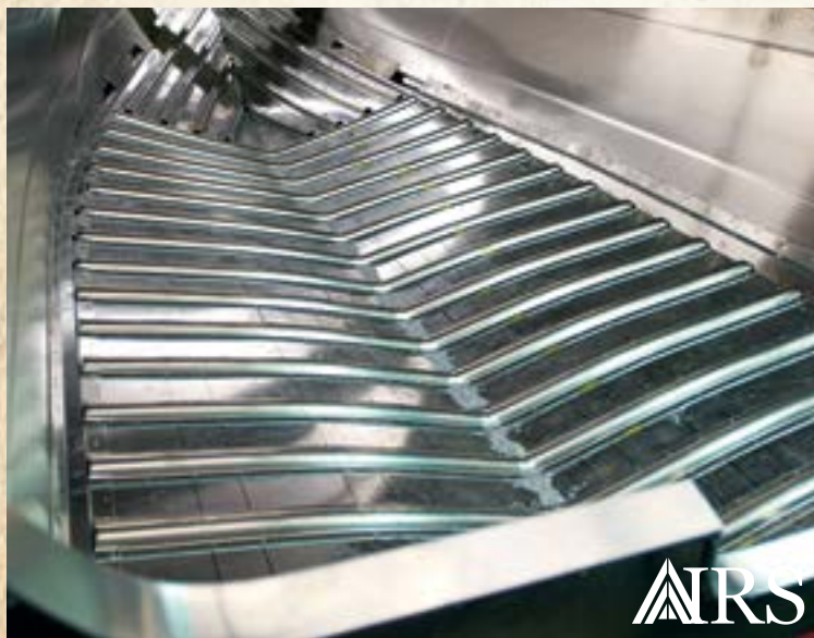
ADVANCED INTEGRATED RIB SYSTEM | hat-shaped ribs on 10" centers, for greater strength and rigidity
