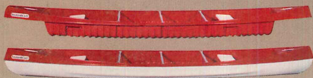
Views showing inner hull above and inner-outer hull joined below
